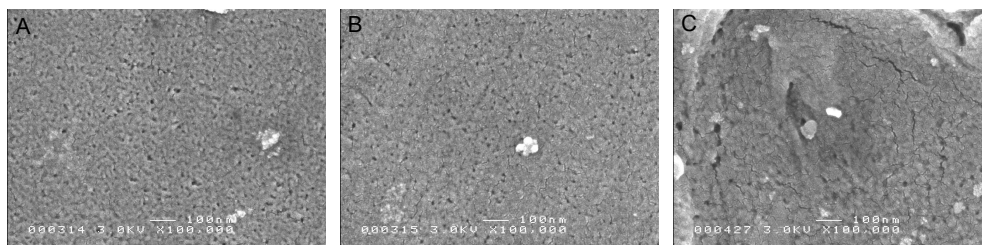
Figure 2.9: The outer surfaces of S1 in the grooves (a) and the fins (b) and the outer surface of R1 (c)
